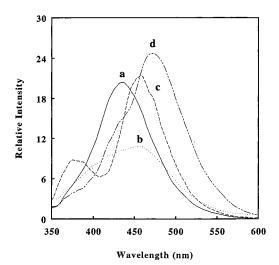
**Figure 4.** Emission of HBO in (a) water (pH 7.0), (b) 8.0 mM  $\beta$ -CD<sub>x</sub>, (c) 8.0 mM  $\beta$ -CD<sub>m</sub>, and (d) 8.0 mM  $\gamma$ -CD<sub>x</sub>.  $\lambda_{exc} = 320$  nm.
