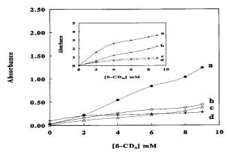
**Figure 2.** Influence of  $\beta$ -CD<sub>x</sub> (0.0–9.0 mM) on the absorbance of (a) MBT, (b) HBO, (c) HBT, and (d) HBI. (inset) Influence of  $\beta$ -CD<sub>m</sub> (0.0–9.0 mM) on the absorbance of the HBA molecules (b–d) and MBT (a).
