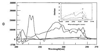
**Figure 3.** Induced circular dichroism (ICD) spectra of  $\beta$ -CD<sub>m</sub> (9.0 mM) with (1) MBT, (2) HBO, (3) HBT, and (4) HBI. (inset) Corresponding absorbance spectra of the molecules in 9.0 mM  $\beta$ -CD<sub>m</sub>, from 240 to 370 nm.
