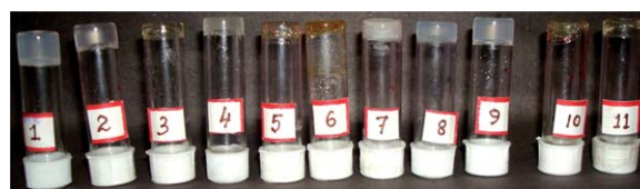
Fig. 2 Gels formed by G-1 : (1) o -xylene; (2) toluene; (3) benzonitrile; (4) chlorobenzene; (5) bromobenzene; (6) iodobenzene; (7) m -xylene; (8) ethyl benzene; (9) p -xylene; (10) nitrobenzene and (11) benzyl chloride.
