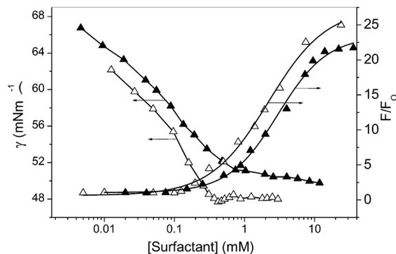
Figure 1. Plots of  $\gamma$  and  $F/F_0$  of AN versus [surfactant] in phosphate buffer (20 mM, pH 7) at 298 K; CS<sub>1</sub> (▲), CS<sub>2</sub> (△).
