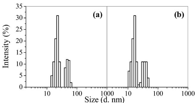
**Figure 4.** Size distributions of SUVs in 2 mM solution of (a) CS<sub>1</sub> and (b) CS<sub>2</sub> in phosphate buffer (20 mM, pH 7).
