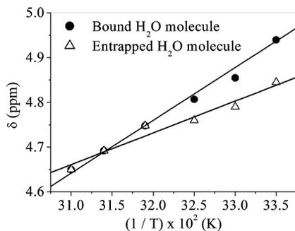
**Figure 6.** Variation of the chemical shift ( $\delta/\text{ppm}$ ) of  $\text{H}_2\text{O}$  with temperature ( $T/\text{K}$ ) in the  $^1\text{H}$  NMR spectra of the  $\text{CDCl}_3$  organogel of **1**.
