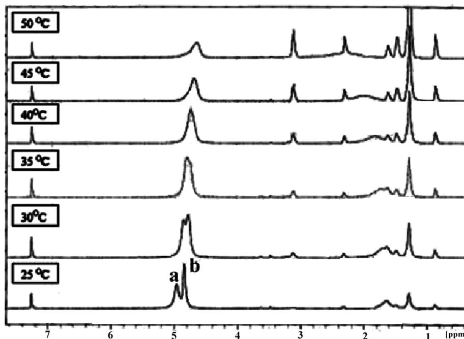
**Figure 5.**  $^1\text{H}$  NMR spectra of organogel **1** in  $\text{CDCl}_3$  containing  $\text{H}_2\text{O}$  at different temperatures. Peak a represents  $\text{H}_2\text{O}$  bound to the urea group, and peak b represents  $\text{H}_2\text{O}$  trapped in the bilayer.
