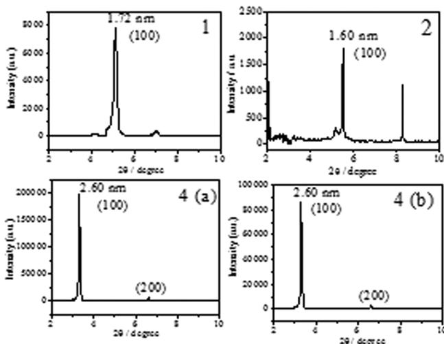
**Figure 2.** XRD spectra of the air-dried organogels of **1**, **2**, and **4** in  $p\text{-Ph}(\text{Me})_2$  at 25 °C. **4 (a)** and **4 (b)** represent the gel made in the presence and absence of  $\text{H}_2\text{O}$ , respectively.
