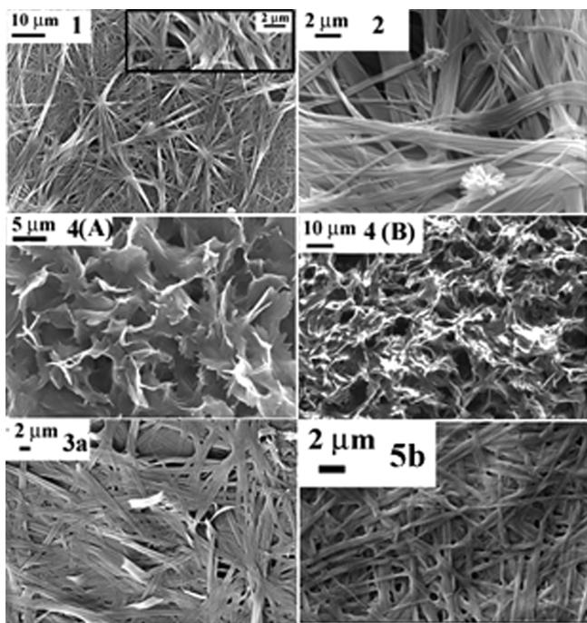
**Figure 1.** FESEM images of the air-dried organogels of **1**, **2**, **4**, **3a**, and **5b** organogels in  $p\text{-Ph}(\text{Me})_2$  at 0.05M. **4(A)** and **4(B)** represent FESEM images of gels formed in the absence and presence of  $\text{H}_2\text{O}$ , respectively.
