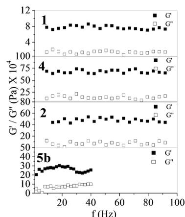
**Figure 3.** Variation of the storage modulus ( $G'$ ) and loss modulus ( $G''$ ) of the **1**, **2**, **4**, and **5b** organogels in  $m\text{-Ph}(\text{Me})_2$  with frequency ( $f$ ) at 298 K.
