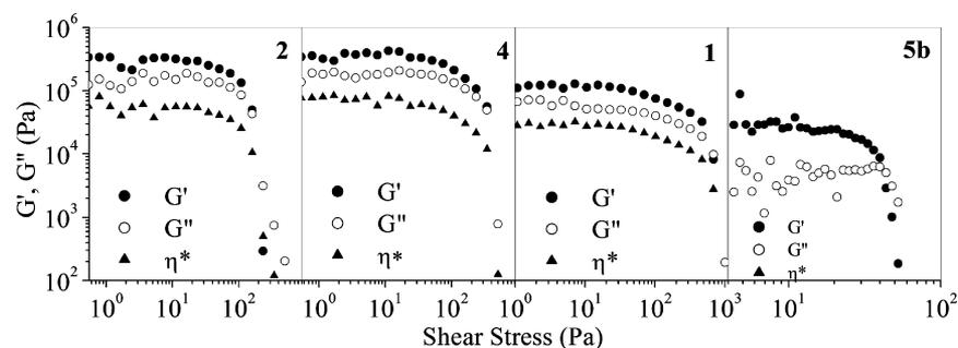
Figure 4. Variation of the storage modulus ( $G'$ ) and loss modulus ( $G''$ ) of the 1, 2, 4, and 5b organogels in  $m$ -Ph(Me)<sub>2</sub> with shear stress at 298 K.
